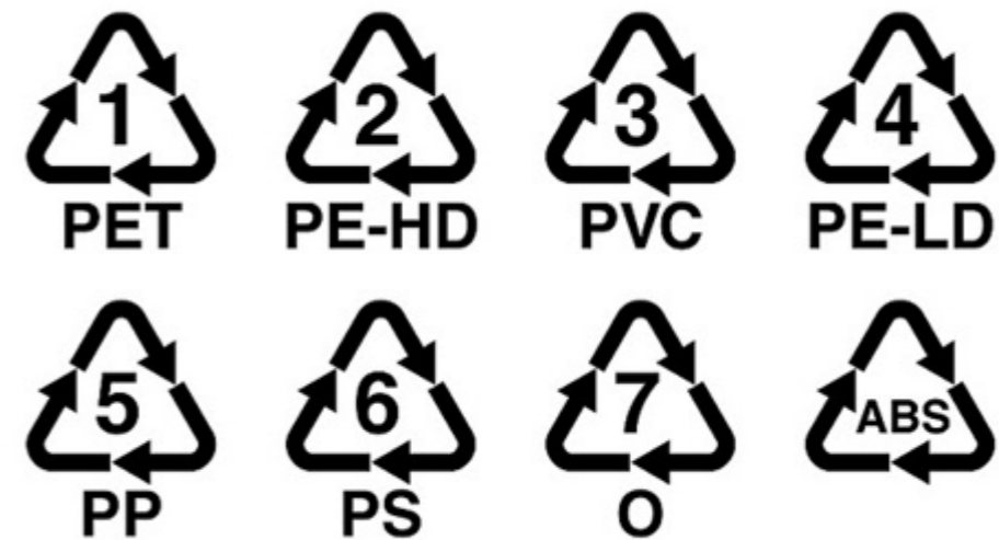
PLASTIC RESIN NUMBERS PHOTO BY CHRISTOPHER VEGA, CREATIVE COMMONS LICENSE: CC BY 4.0
