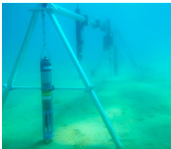
Figure 8: Sediment resuspension device. UC Davis
